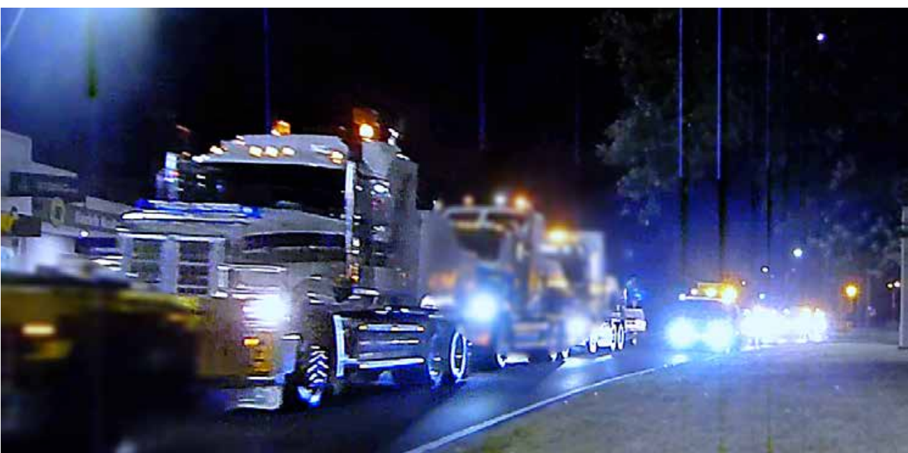
Three trucks pushed and two pulled to move this 650 tonne superload. Image; Trevor Colvin
