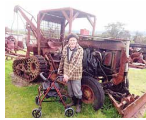
Hank repurposed this Bren Gun carrier to drag sawlogs from the bush.
