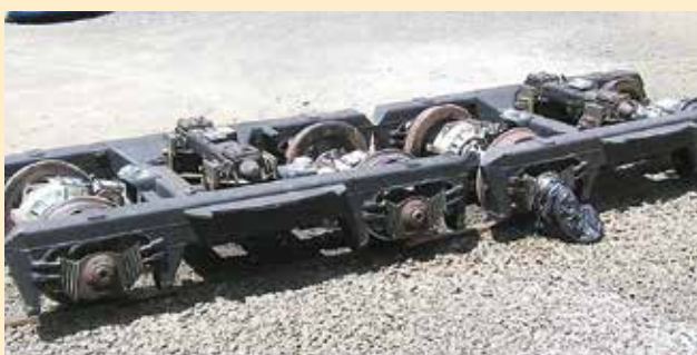
The rail motor has been regauged with new bogies
